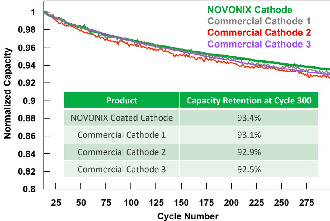
40°C; 2.8-4.3V; 1.2M LiPF<sub>6</sub> EC:EMC:DMC(25:5:70)+3VC; [Charge] : CC-0.33C; [Discharge] : CC-0.33C
