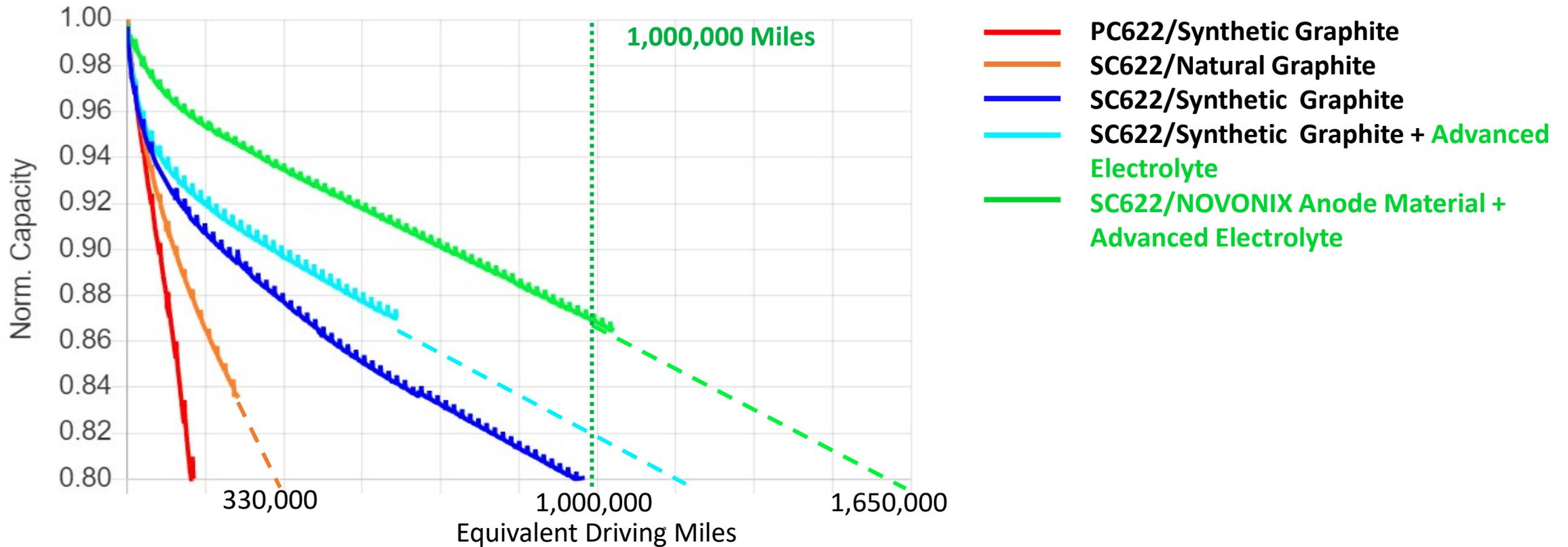
Building full cells for performance testing to demonstrate performance of NOVONIX anode, cathode, and electrolyte technologies in a single cell
