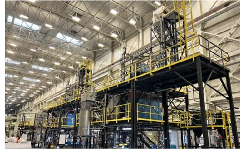
NOVONIX Generation 3 Continuous Induction Furnace Systems
